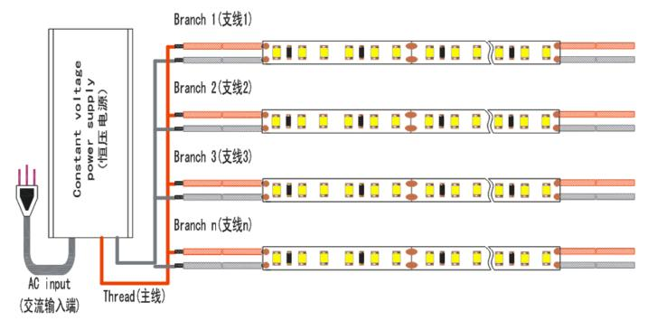
Note:To achieve better luminous effect, it's suggested that the power supply cable of each 5 meters long lamp should be connected to the power line.
